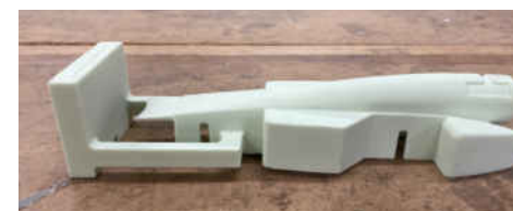
» Car milled from foam block using new machining plan, without defects. Credit: Hydron
