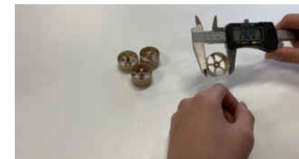
✖ Checking dimensions of PEEK wheels from ArpTech, measuring a 28.2mm diameter exactly as designed. Credit: Hydron
