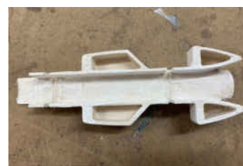
» Test balsa milled car, with machining errors on sidepod and in central tunnel. Credit: Hydron
