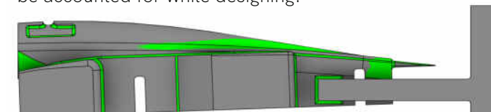
✖ Fusion 360: Minimum Radius Analysis of 1.5mm, ensuring that all concave parts of the car would be accessible to a 3mm ball nose endmill. Credit: Hydron
