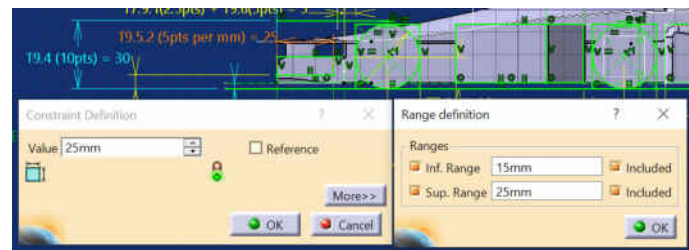
✖ CATIA v5: A limited dimension, ensuring that the front wing remains in a legal location. Credit: Hydron
