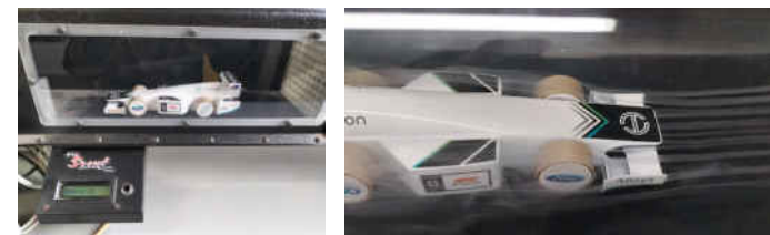
✖ Final car airflow structure verification using smoke in wind tunnel. Credit: Hydron
