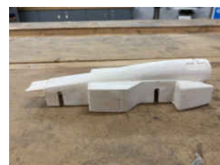
» Test balsa milled car, with machining errors on sidepod and in central tunnel. Credit: Hydron
